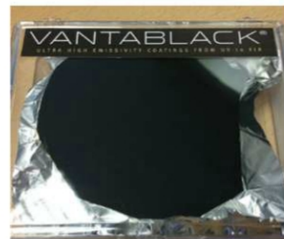
Via its system of carbon nanotubes, Vantablack absorbs 99.96 percent of light.
