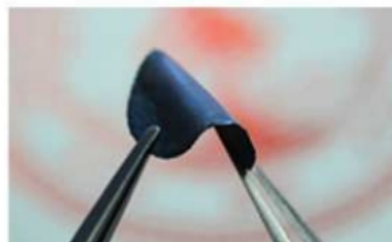
This carbon nanosphere film guards the lithium battery's anode from harmful chemical reactions that would render the high-energy battery useless.
