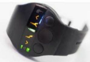
Wrist device commands the exoskeleton to sit, stand or walk
